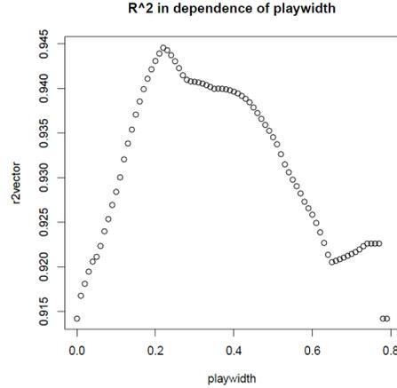
was created under the assumption of a constant play of 0.22, that is we assume that changes smaller than 0.22 are ignored. This play width was estimated and reflects the one for which the addition of the respective spurt is able to improve the regression most. The spurt series is more stepwise and reflects a broader filter than the Preisach hysteresis variable.
