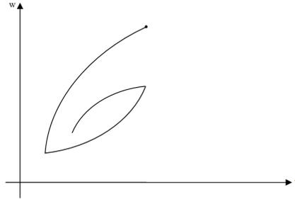
Aggregation of many of these non-ideal relays with different threshold values results in a hysteresis loop, see Figure 2.
